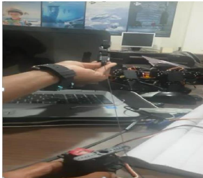
Single DoF finger actuated by servo motor.
