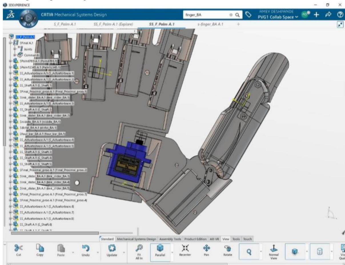
Thumb assembly and actuation on servo motor
